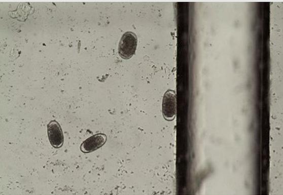
On each individual sample, FEC will be performed to obtain worm EPG (eggs per gram of faeces) data using a quantitative copro-microscopic method e.g. Mini-FLOTAC, McMaster, FECPAKG2 etc. using saturated sodium chloride (specific gravity = 1.200) as flotation solution. When low number of eggs are expected sensitive methods are recommended (e.g. Mini-FLOTAC, analytic sensitivity of 5 EPG) (Cringoli et al., 2017).
